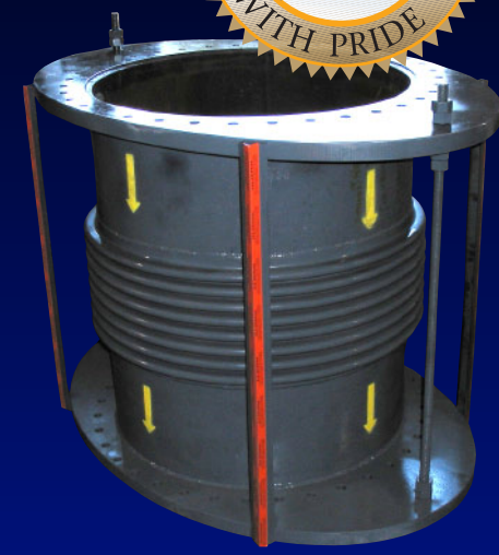
Custom Designed Joint: 30" nominal ID x 36" Fx F, expansion joint with stainless steel liner. Custom elliptical steel flanges, 35" x 50 Fx F" with control rods. Design 150 psi @ 650°F
